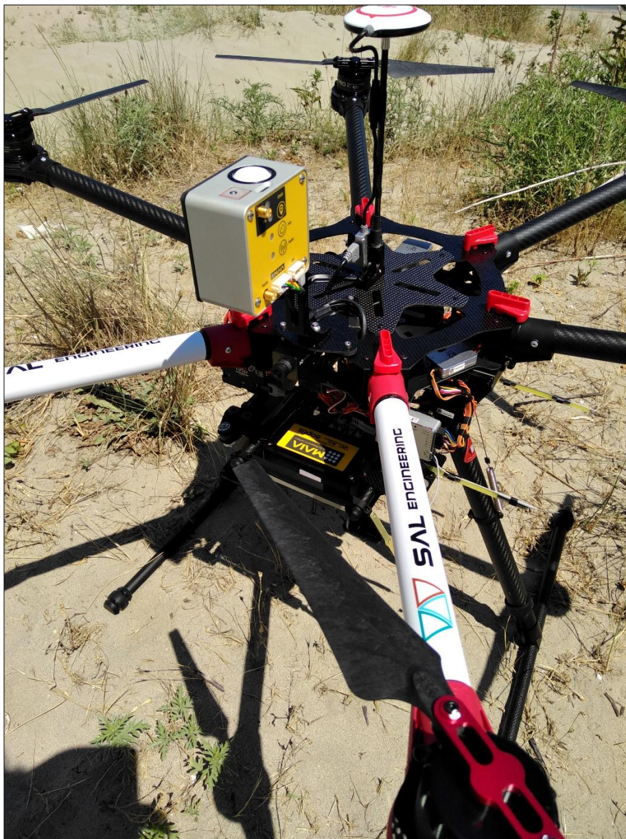
Figura 4 ILS mounted onboard a RPAS in connection with MAIA multispectral camera.
